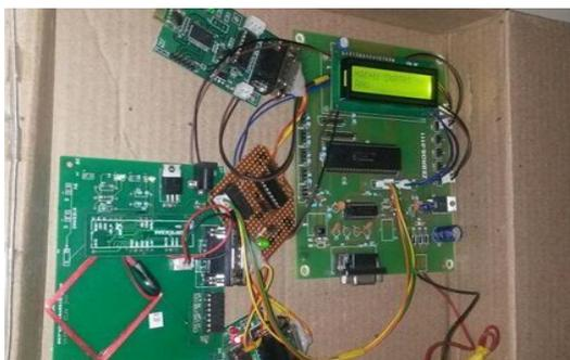
One side of the module contains the biomedical sensors to sense the various parameters and the other side sends the data to the imed box module through Zigbee. A buzzer is also connected to alert the patient to take medicine at proper time.
